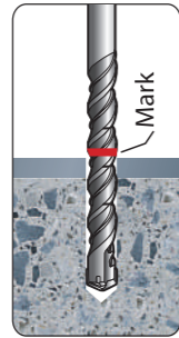
Khoan lỗ Drilling hole with Recommended Diameter And Depth
