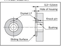
**%** Sliding surface consists of a plastic layer.
