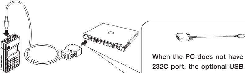
When the PC does not have any RS-232C port, the optional USB-RS232C converter is necessary for our specifications to VZC-53 and the PC.
