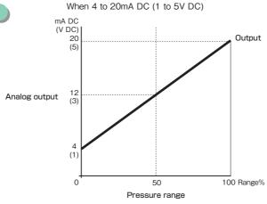
Output is linear to 4 to 20mA DC (1 to 5V DC) against rated pressure range.
