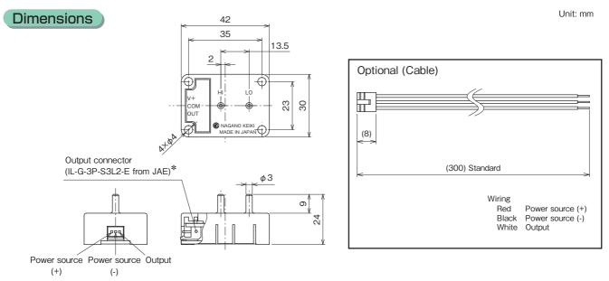
\*For the mating connector, use type IL-G-3S-S3L2-E from Japan Aviation Electronics Industry, Limited (JAE)
